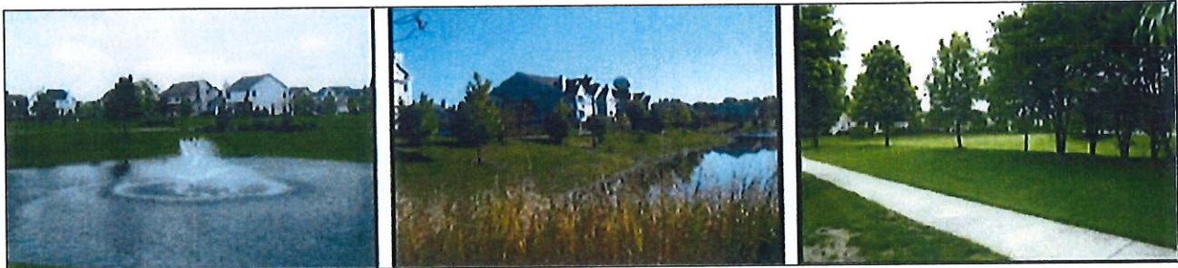
A pond can be an amenity to a neighborhood. The pond on the left incorporates a fountain feature, whereas the center pond uses native plantings as a means to enhance its perimeter. The dry bottom pond on the right, provides an open area for activities such as unstructured ball games (i.e., soccer, baseball), kite flying and family picnics.
